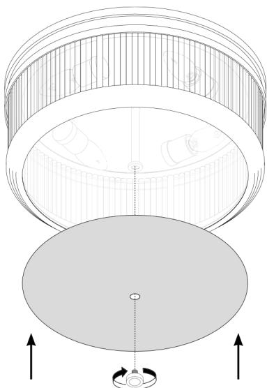
Turn off the electricity supply at the main circuit panel before installing. Do not connect the electricity supply until your luminaire is fully assembled and installed.
